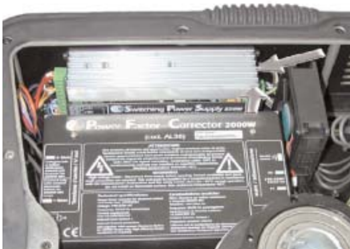
Figure W11C- Removing Switching Supply
